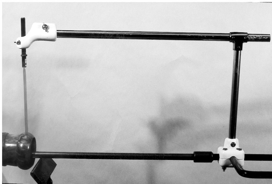
The author's laser system, above. As the tool moves, the laser moves in the same way. The beam is set to desired wall thickness, as shown at top left. When the desired thickness is achieved, beam slips off vessel, as shown at lower left.
