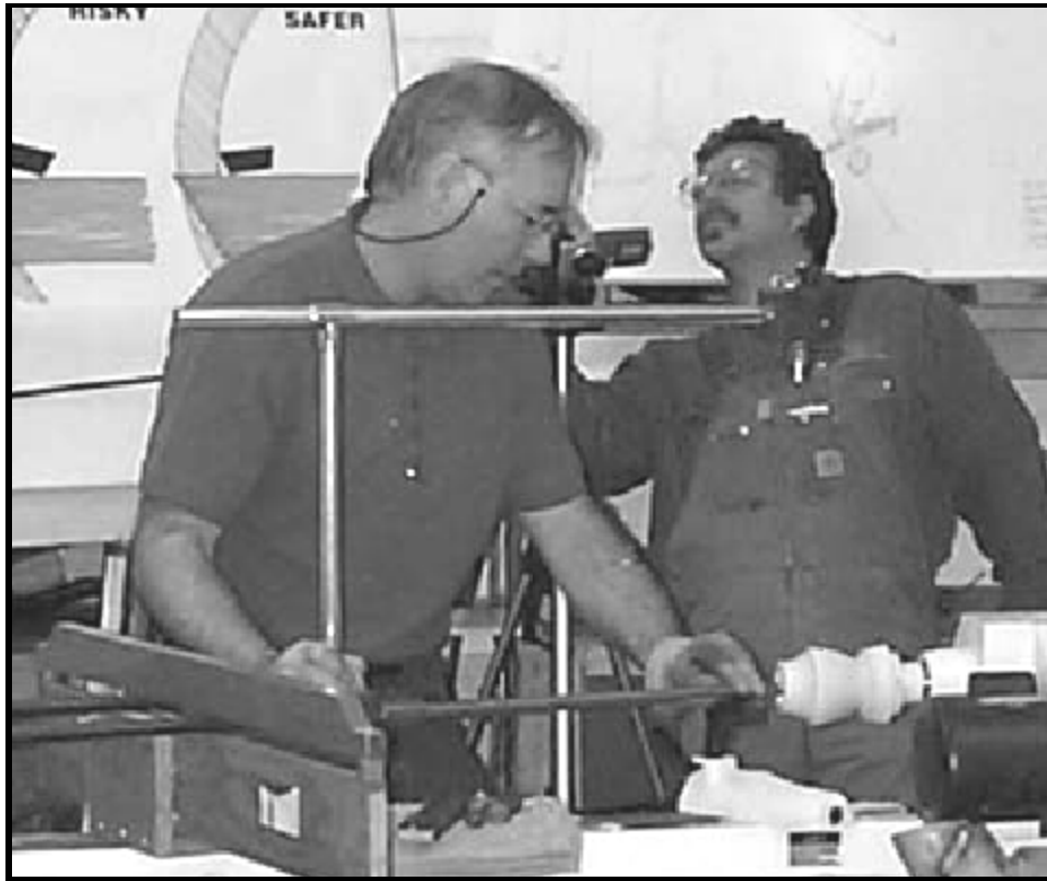
Lyle Jamieson with his boring bar and laser wall thickness measuring device shows how easy it is to hollow a form and get the desired wall thickness.
