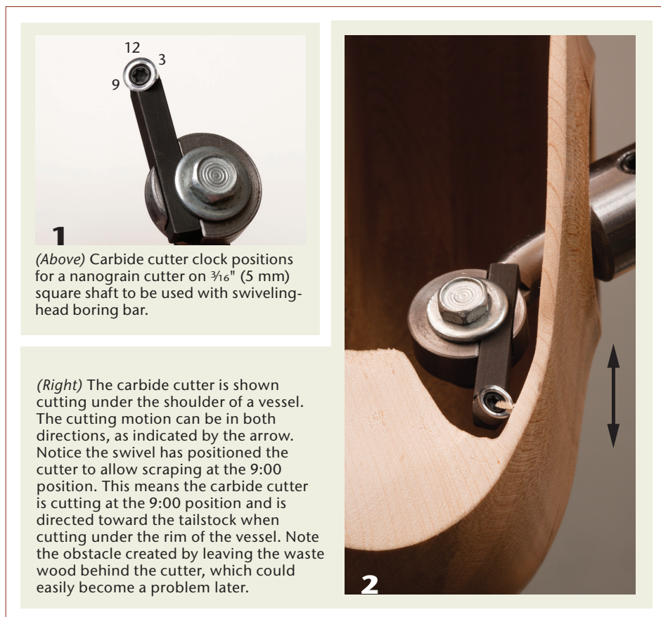
Figure 2. Nanograin carbide cutter in three positions tilted to cut wood (or not).
