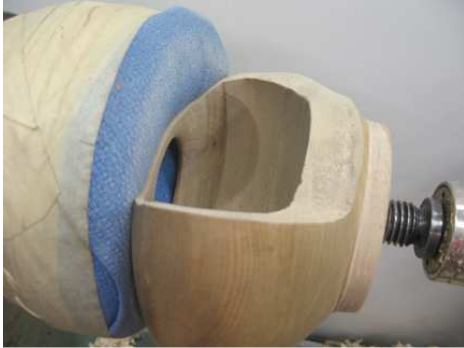
Shows cut away hollow form reversed in "donut" with cloth padding taped on it to protect vessel wall.
