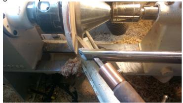
The bar holds the tool high enough that I can leave it in its handle and not interfere with the tool rest, so that I can keep the support as close to the cut as possible.
