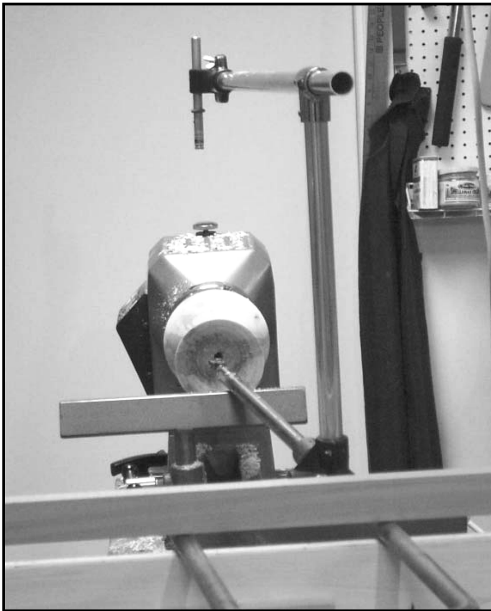
This view cleans up the background a bit and gives a better view of the laser pointer and its mounting fixture.
