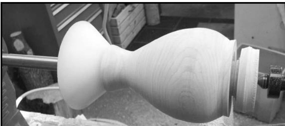
The San Diego Woodturners came up with this mounting for reverse turning a hollow vessel. I'm not sure whether they are commercially available at this time or not. I purchased one of the overrun that they ordered when getting them made for their club members.
