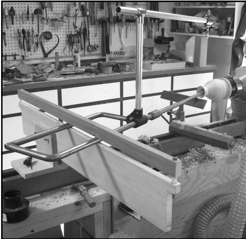
Here the Lyle Jamieson boring bar with laser pointer attachment is shown set up on my Nova DVR 3000. I had to add a bed extension to make my lathe long enough to use the rig. Lyle sells the boring bar and laser attachment and you make or buy the rear tool rest. I'm using the one that came with my boring bar from Turningways.
