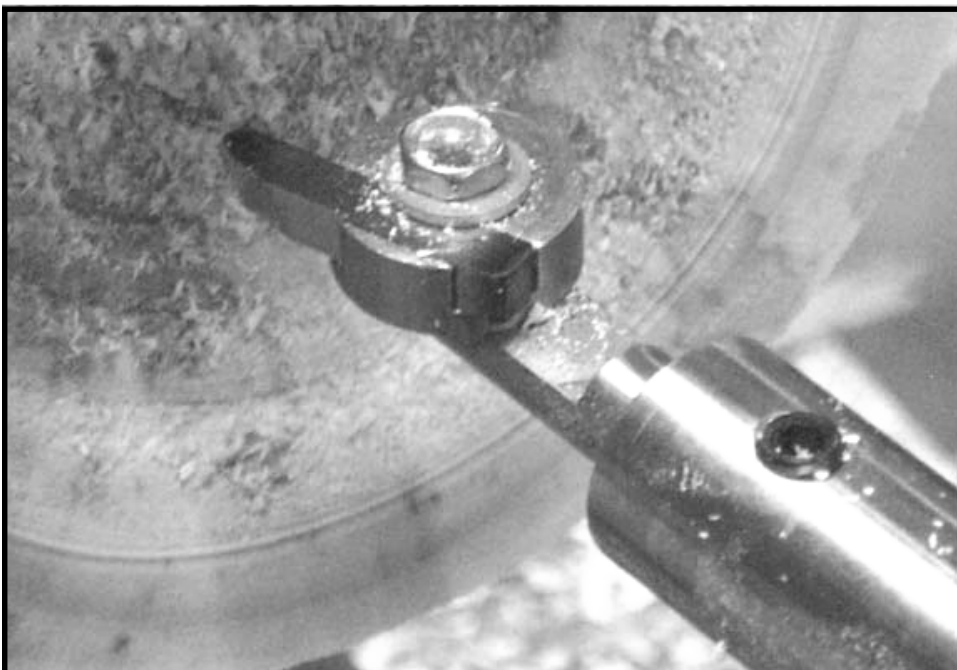
The cutting head may be rotated to any angle that seems appropriate for the particular cutting task.
