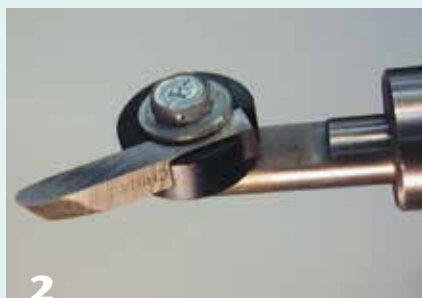
2 A swivel assembly with HSS cutter. Note the grind on the left side of the cutting tip. This grind configuration allows ease of cleaning up tool marks.
