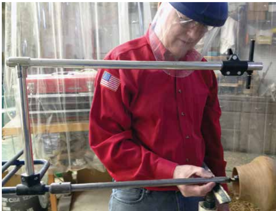
A proper captured hollowing system allows you to turn inside the hollow form with only fingertip control. Note my body position and stance; it should not be hard work.
