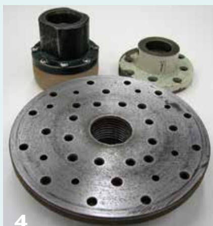
4 Both the large 7" (18cm) faceplate and smaller glue-block faceplates have been upgraded by drilling additional screw holes. Precise placement of the holes is not necessary. A 4" (10cm) faceplate with 12 holes (not pictured here) is sufficient for safely attaching a log for hollowing.
