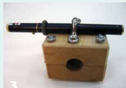
3 A simple bracket will clamp the laser to the support bar.
