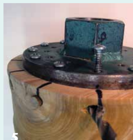
5 When screwing into endgrain, dowels inserted perpendicular to and aligned with the screw holes will greatly increase holding power. Drill deep into the wood so the screws go through the dowels.
