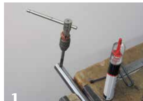
1 While tapping threads, the hole size has to be precise to allow the tap to cut cleanly and accurately.
