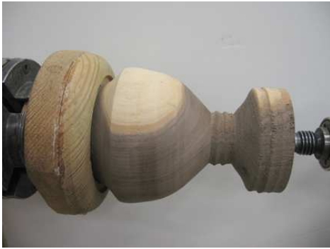
Shows walnut hollow form with solid rim recessed into waste block.
