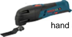
light force and move around a little. Lay the blade flat on the surface. After the first couple you can almost do a perfect job just with the saw with only hand sanding left.
