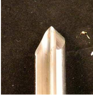
This is the photo of Stuart's gouge and the incorrect grind
